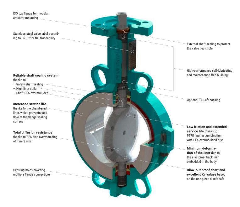
The high liner collar, the PFA disc overmoulding on the shaft as well as a life-time preloaded safety shaft sealing guarantee both excellent primary and long-lasting secondary shaft sealing, even for greater operating cycles and at high temperatures.
