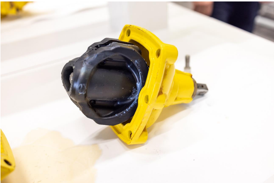
Figure 7 No visual internal damage present on either valve type.
