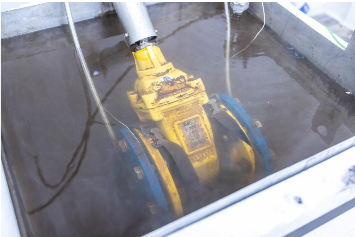
Figure 2 Valve placed in water bath post function test, prior to burst test.
