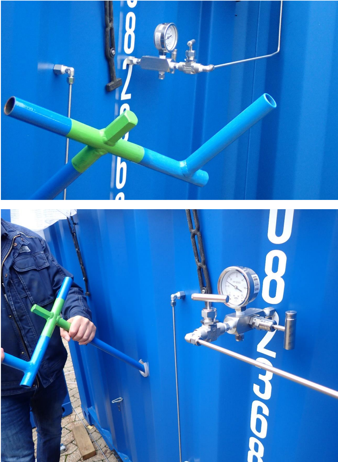
Figure 3 Function test of 200 cycles conducted through handle outside the container.
