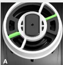
If the valve is over torqued, the topcap is designed to fail before the valve seals, thus preventing a leak to atmosphere. The **safety topcap** can be replaced easily under live conditions.
